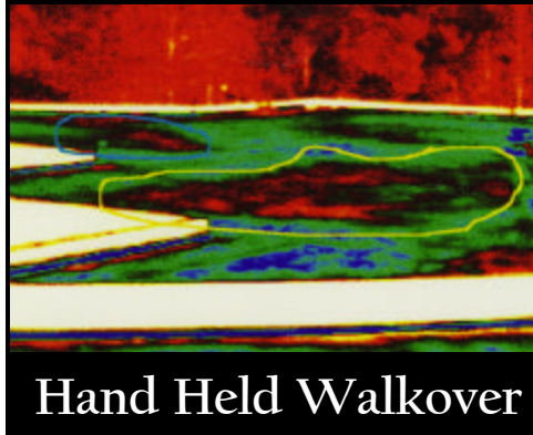
Walk-over infrared inspections became available over a decade ago. The image above represents one of 100's of photos which must be captured at less than a 60 degree angle to provide full roof documentation. This documentation is subjective and often misinterpreted.
