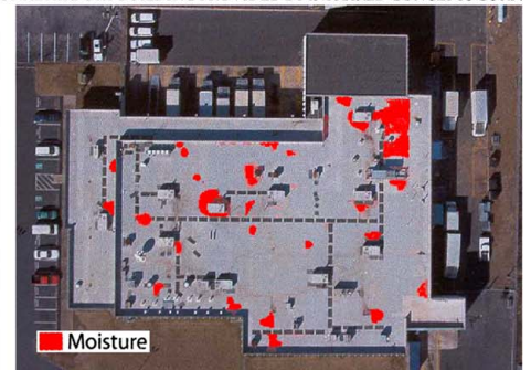
4) Superimposing the computer image on the daytime photograph, using red ink to show possible leaks.
